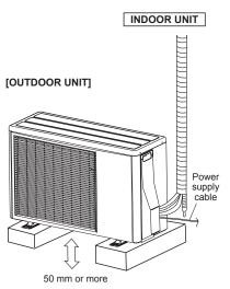
Do not install directly on the ground, this may result in equipment failure. Make sure the height of the base is 50 mm from the ground.
