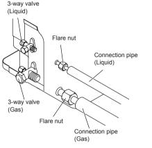
(4) When the flare nut is tightened properly by your hand, use a torque wrench to finally tighten it.
