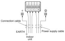
(5) Power supply cable and connection cable should be fixed with cable clip as shown in the figure.
